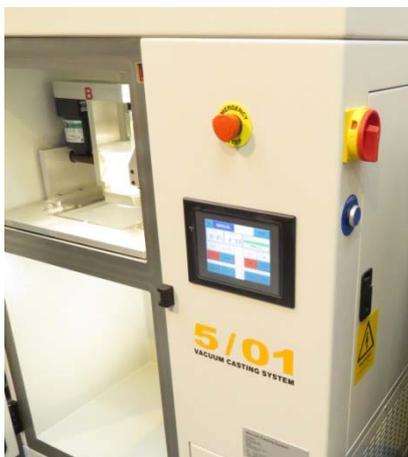
Figure 11A Turn isolator and E-stop off
