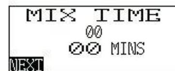
Enter key to accept this time. As the user enters the numbers, these will be displayed in smaller numbers and then when Enter is pressed will be transferred to the larger numbers.
